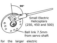
Alternatively you may choose to place the ball link at a distance that allows the servo to have a combined travel of around 80° from the low endpoint to the high endpoint.
